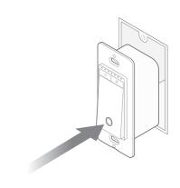
Attach the wallplate and turn on the circuit breaker. Then the wiring is finished.
