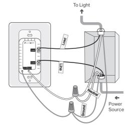
5 Line up the dimmer switch with the mounting holes. Secure it with secret mounting holes. Secure it with screws.
